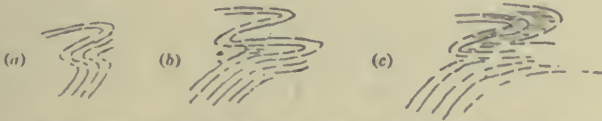
FIG. 86.—FOLDING OF FOLIATION OF FISSILE BED AT JUNCTION WITH OVERLYING GRIT. Cliff north-north-east of Maen-y-fran, Rhoscollyn.
